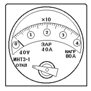
Fig.14. Voltage & Current Indicator (ИНТ)
