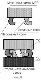
After the spacecraft/station structural latching and alignment the spacecraft active hooks are positioned opposite the station passive hooks and the station active hooks opposite the spacecraft passive ones.
