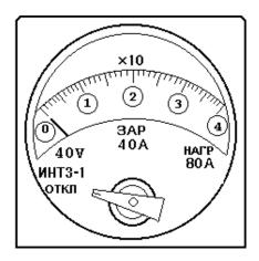
Fig. 11. Voltage & Current Indicator
