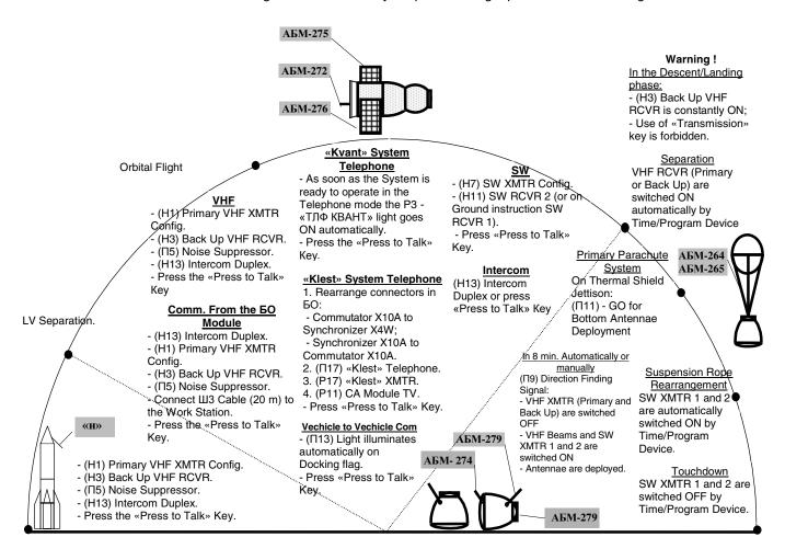
Fig. 3. (Soyuz Spacecraft Flight Phase Communication Arrangement)
