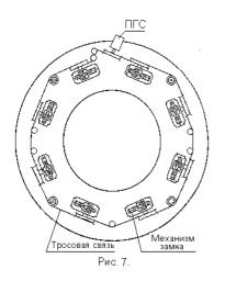
The **MFC** (Interface Pressurization Mechanism) is designed to ensure the second mechanical link, i. e. rigid and hermetically sealed connection of the spacecraft and station docked. The design of the ACA (Active Docking Assembly) MFC and the FICA (Passive Docking Assembly) MFC is identical. The MFC consists of:
