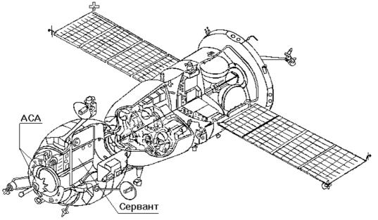
Fig. 2. (Spacecraft CCBI Main Element Location)
