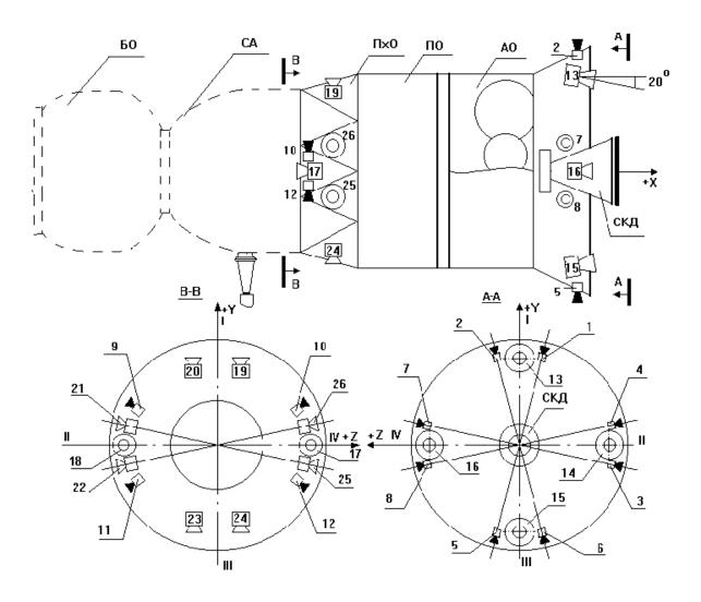
Fig. 1. (КДУ Thruster Location Layout)
