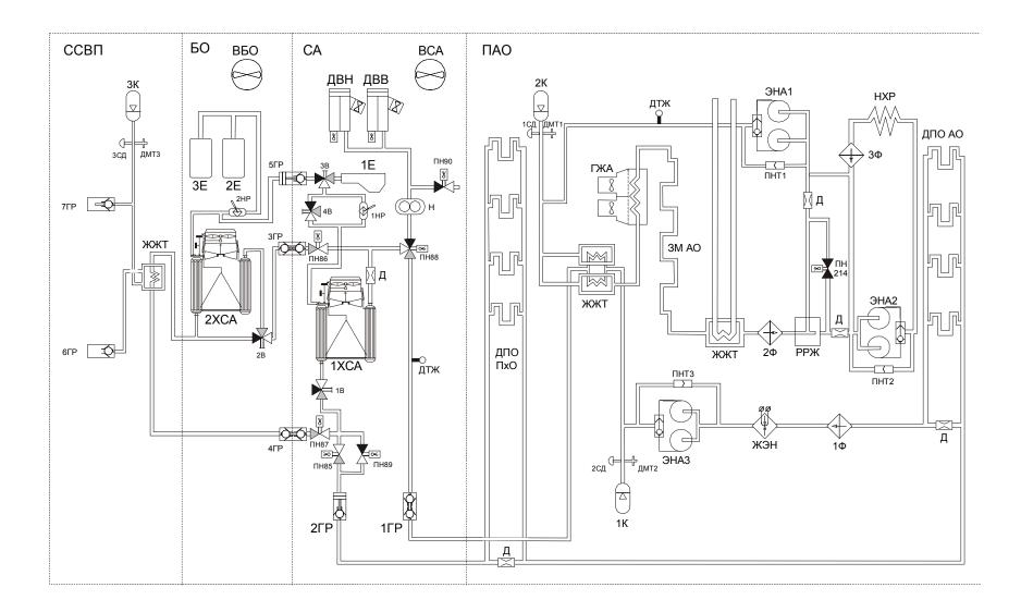
Fig.1. Soyuz TM Spacecraft CTP (Thermal Control System) Functional Block Diagram
