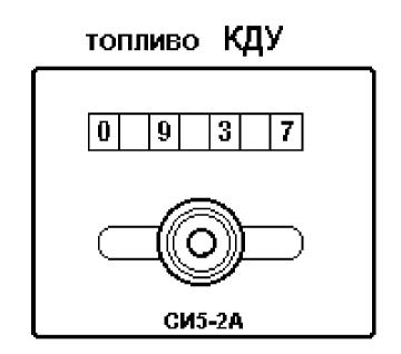
Fig.9. Propellant Quantity Meter (СИ)
