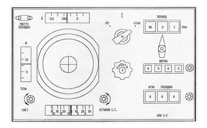
Fig.8. Space Navigation Indicator (ИНК)
