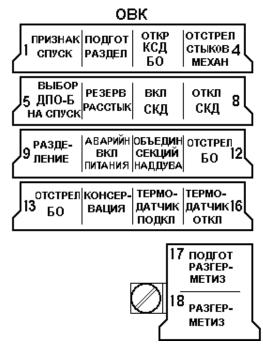
Fig. 7. OBK (Critical Command) Keys
