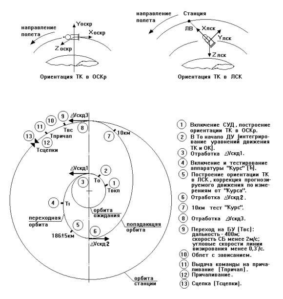
Fig. 2. (Spacecraft to Station Approach Cyclogram)
