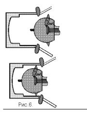
In the forward part of the CM Rod there are four Latches. The Latches can be in either of the two positions: extended or retracted, the extension and retraction being executed by the latch retraction mechanism driven by the Latch Actuator ( $\Pi$ 3).
